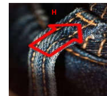
H - Bolt stitching on both seam ends
